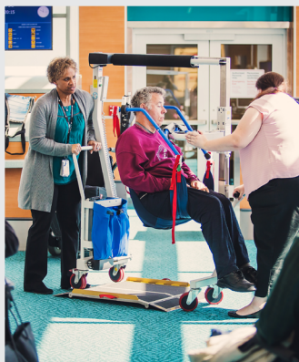
3) Lift fits over aircraft seat and lowers passenger into their seat.
