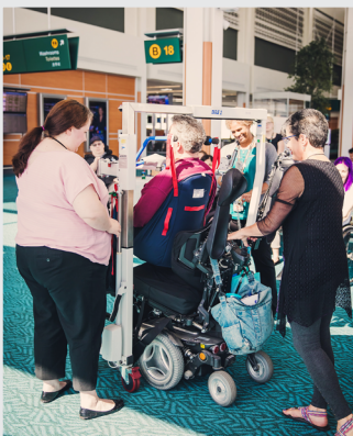
2) Powered lift elevates sling and user.
