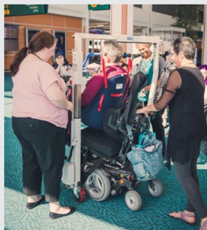
2) Powered lift elevates sling and user.
