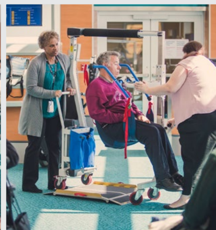
3) Lift fits over aircraft seat and lowers passenger into their seat.
