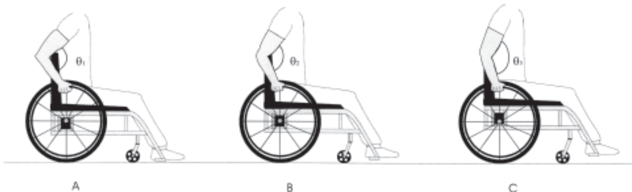
FIGURE 2: ILLUSTRATIONS A-C SHOW DIFFERENCES IN THE ELBOW FLEXION ANGLE ( \theta ) FROM ADJUSTING THE HEIGHT OF THE AXLE. ILLUSTRATION B DEPICTS THE RECOMMENDED ELBOW ANGLE ( \theta_2 = 100 TO 120 DEGREES). ANGLE \theta_1 IS SMALLER BECAUSE THE SEAT IS TOO LOW (AXLE TOO HIGH). ANGLE \theta_3 IS LARGER BECAUSE THE SEAT IS TOO HIGH (AXLE TOO LOW).
