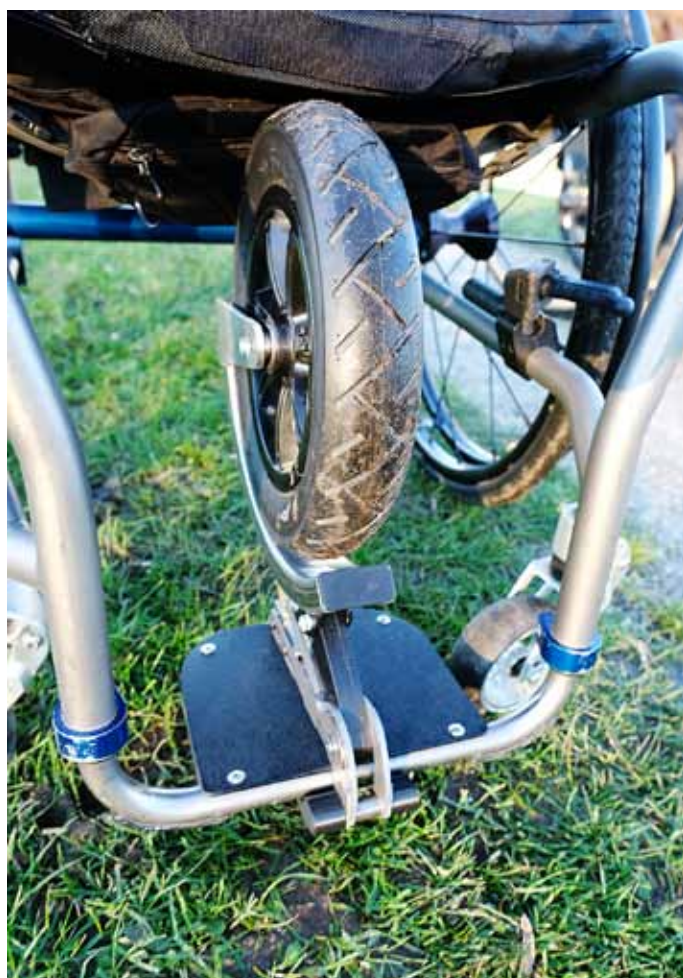
LEFT: When not needed, the SWIVL rotates up and in, and stores between the user's legs. RIGHT: When required, it rotates out and down, where it locks securely into place. It takes seconds for the user to switch from one position to the other.
