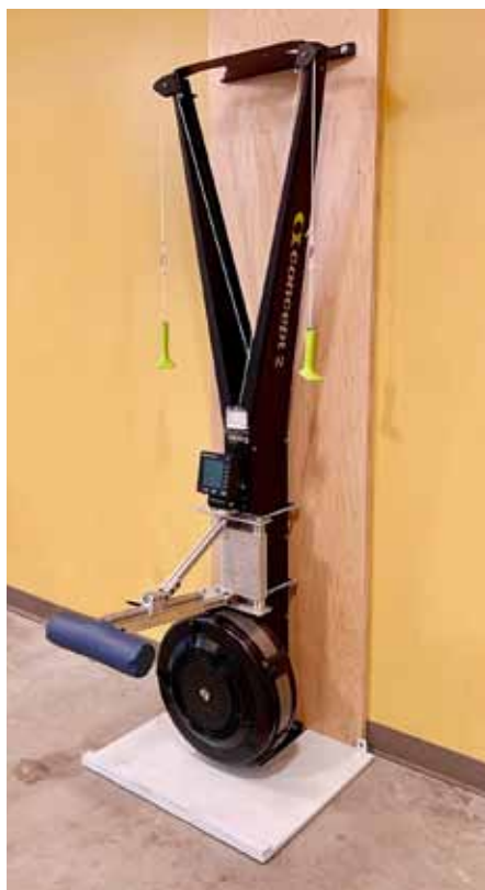
The Concept 2 ski ergometer can be used out of the box by some people with SCI, but the aSKI modifications (such as the lap brace shown) make it even more accessible.
