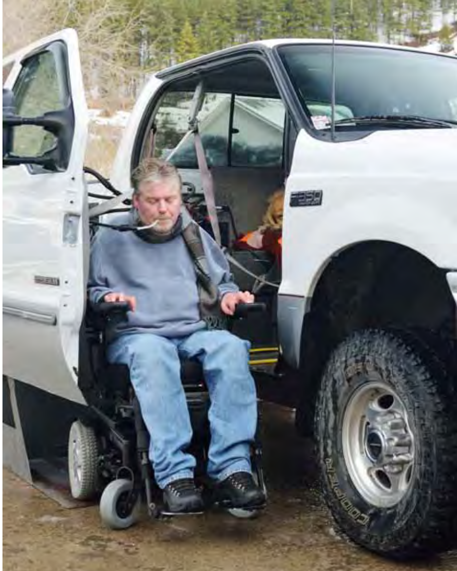
READY FOR THE BACKCOUNTRY: The lift built by Swanson's father is truly a feat of DIY engineering. Swanson first wheels backwards into the lift as it rests on the ground (left). He's then lifted vertically (top right), and then moved horizontally into the cab of his Ford F350 4x4.
